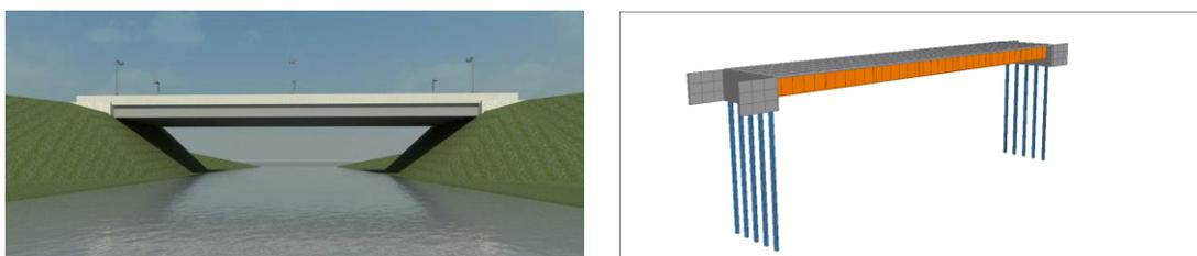
Figure 3: Simple Span Bridge and 3D Finite Element Model
