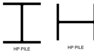
Figure 3: HP Steel Pile
