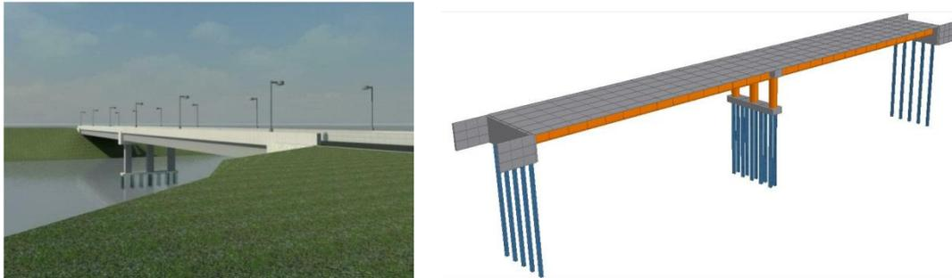
Figure 4: Two-Span Bridge and 3D Finite Element Model
